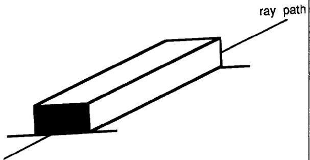
Figure 1: Natural pixel for a single ray.
