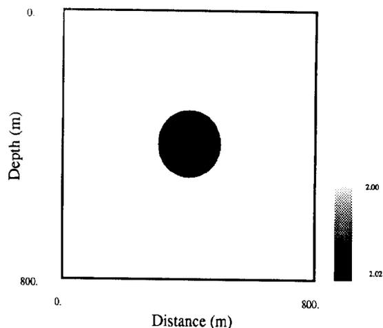
Figure 3: Slowness perturbation. 17 sources are located on the right hand side of the model and 17 receivers are located on the opposite side. The radius of the disc is  $r = 100\text{ m}$ . The width of the natural pixels is  $\lambda' = 40\text{ m}$ . The vertical separation between adjacent sources and/or receivers is 50 m.
