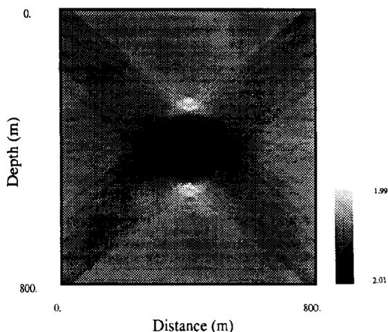
Figure 5: Inversion when the model is discretized in natural pixels. The image is displayed in a grid of 161 X 161 cells.
