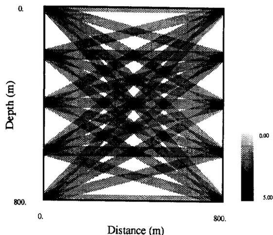
Figure 2: Natural pixels in a constant slowness medium for a cross-well configuration of five sources and five receivers.
