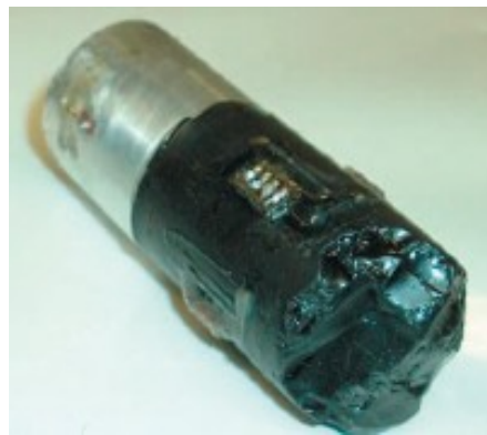
Figure 3.10. Heavy oil (GP007-Uvalde) sample with semiconductor strain gages attached to the surface (from Behura et al. 2007)
