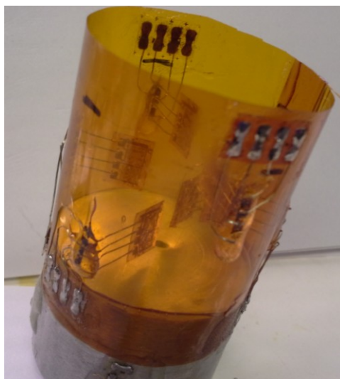
Figure 3.11. Example of jacket design to measure elastic properties of soft samples. The jacket is made of kapton which is resistant to heat and flexible enough to allow deformation of the soft sample. The jacket is attached to an aluminum standard, six pair of gages, three vertical and three horizontal are inserted in the jacket.
