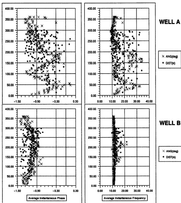
Figure 2. Comparison of variability of two seismic attributes around wells A and B at Lake Maracaibo. Note dispersion in well A.
