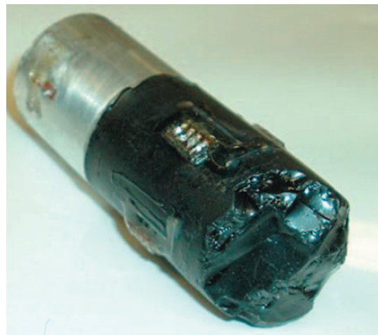
Figure 3. Heavy-oil (GP007-Uvalde) sample with semiconductor strain gauges attached to the surface (from Batzle et al., 2006b).
