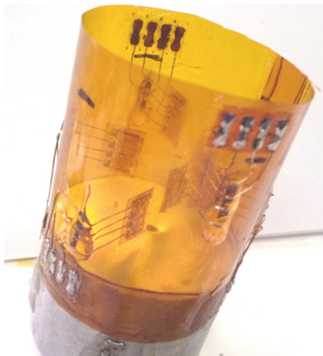
Figure 4. Example of jacket design to measure elastic properties of soft samples. The jacket is made of Kapton, a material resistant to heat and flexible enough to allow deformation of the soft sample. The jacket is attached to an aluminum standard with six pairs of gauges, three vertical and three horizontal, inserted in the jacket. The jacket used for the experiment shown in this work had outside gauges attached to the surface of the jacket.
