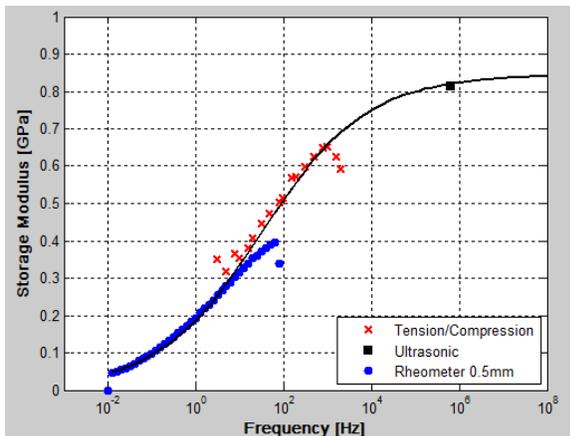
Figure 5. Shear modulus ( $G'$ ) vs. frequency (Hz) for the GP007 sample, using three techniques and 0.5 mm “confined” gap thickness. Tension/compression and ultrasonic data from (Batzle, et al. 2006b).
