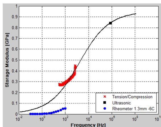
Figure 1. Storage modulus ( $G'$ ) vs. frequency for sample GP029 from different techniques and Cole-Cole model. Rheometer data was measured at 1.3mm gap thickness ("bulk").
