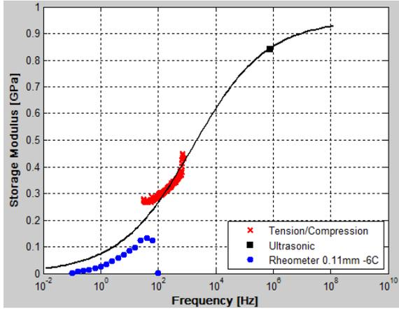
Figure 4. Storage modulus ( $G'$ ) vs. frequency for sample GP029 from three different techniques and Cole-cole model. Compared to the rheometer results at a small “confined” gap (0.11 mm).
