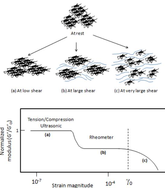
Figure 3. Schematic representation of heavy oil behavior under shear at different amplitudes. Upper image shows a representation of the molecular behavior, and the lower image shows the corresponding expected shear modulus with strain amplitude.
