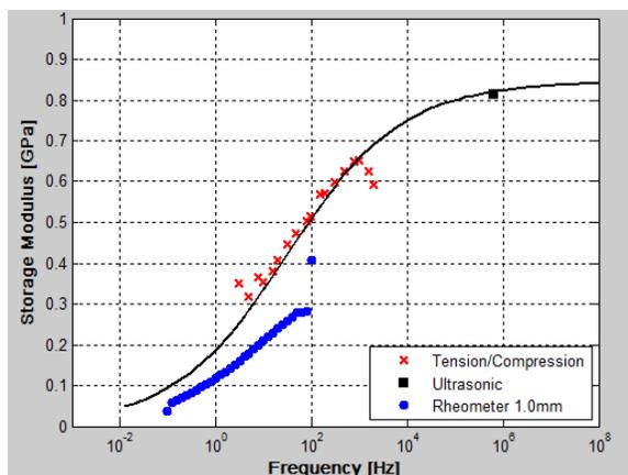
Figure 2. Storage modulus ( $G'$ ) vs. frequency for sample GP007 at 1 mm gap thickness ("bulk") for the rheometer results.
