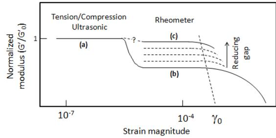
Figure 6. Modification to Figure 3 adding the appearance of an “equivalent” solid-like LVR (c) with the rheometer after reducing the gap thickness.
