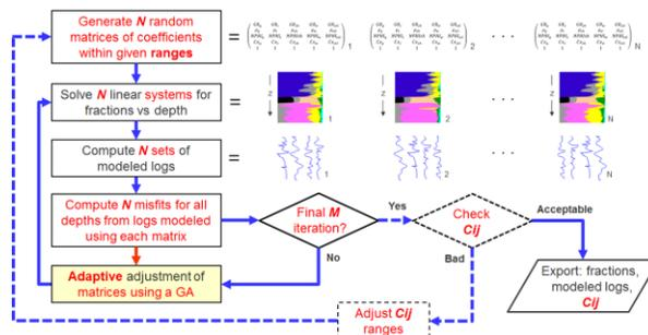
Figure 2. Nonlinear multiminereral analysis to estimate fractions and mineral constants. Different matrices of constants are adjusted automatically until an acceptable match is obtained.
