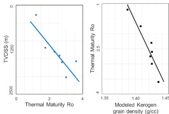
Figure 5. Thermal maturity from vitrinite reflectance  $R_o$  for the Marcellus Formation. Left: Variation of  $R_o$  vs depth. Right: Correlation of modeled kerogen density vs  $R_o$ .
