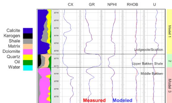
Figure 3. Result of multiminerals analysis in the Bakken Formation. The good agreement between measured (red) and modeled (blue) logs indicates that the estimated fractions and mineral constants are plausible.
