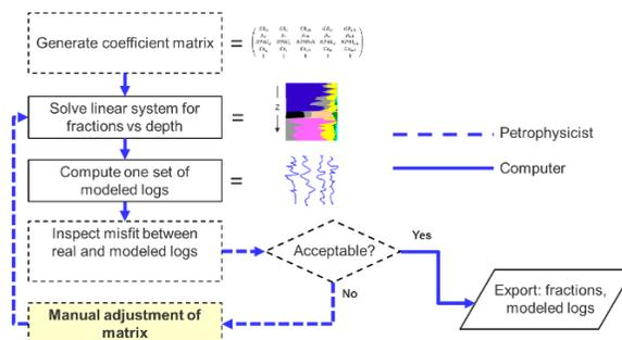
Figure 1. Conventional multiminereral analysis to estimate fractions of constituents. The matrix of mineral constants is adjusted manually by trial-and-error until an acceptable match is obtained.
